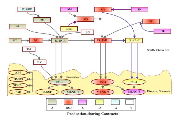
Figure 2-4: The Sarawak Gas Production System: Network overview (not to scale)
