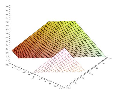
Figure 2-2: The feasible region of QP subproblem at (5,4,3) is intersection of the two parallel hyperplanes resulting in an empty feasible set
