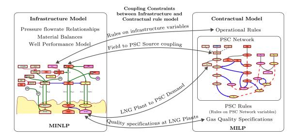
Figure 2-5: Upstream planning model: Overview of components
