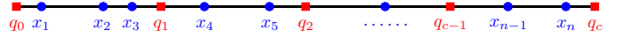
Fig. 1. Geometry of the charged particles and the control electrodes along a line segment. The disks represent the particles while the boxes stand for the electrodes.
